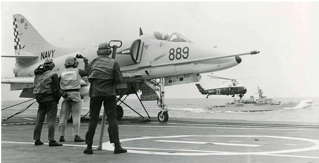
Skyhawk 889 which was lost on 8 November 1973 after a failed catapult launch. The shuttle is just behind the nosewheel, with the bridle being the two taut wires leading from it to the catapult hooks in the mainwheel wells. The holdback is the taut wire under the flaps at left, with the holdback restraint the two loose cables under it. The Flight Deck Officer is waving his green flag in his right hand. (FAAAoA)
