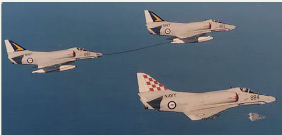
Two VC724 A-4s practice air-to-air refuelling with a VF805 Skyhawk alongside. (Peter Greenfield)
